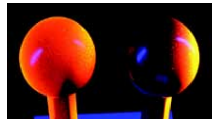
In the above test fluorescent dye has been sprayed on two round knobs. The left knob was sprayed with the electrostatic system ON; the right knob was sprayed with the same applicator, but with the electrostatic system OFF. Note how even the coverage is on the left knob with electrostatics ON.
